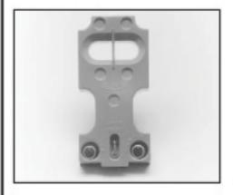
The logic module interconnects the power block and scanner block both electrically and mechanically using a unique blade-and-socket connector concept. It also provides the LIGHT/DARK operate function (except in the LM1) and the timing functions, all of which are fully adjustable.
